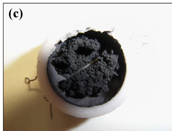
Fig. 12. Anode surface of cells after poisoning test (poisoning 200 h) by mixing with (a) 3% C_2H_6 and 3 ppm H_2S , (b) 3% C_3H_8 and 3 ppm H_2S , and (c) i-C_4H_{10} and 3 ppm H_2S , revealing severe accelerated carbon deposition.
